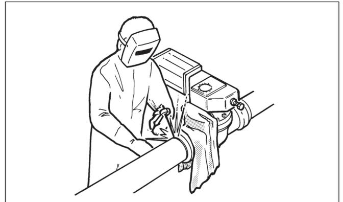
Fig. 6 Valve body covered with wet protection cloth during welding
