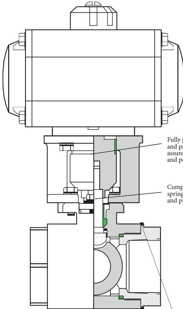
Fully guided stem, coupling and precision bracket assures optimum form, fit and performance
