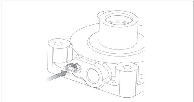
To achieve perfect cushioning, ensure cushioning screw is full open at the time of installation. Operate cylinder in full forward to full back. Now keep on tightening cushioning screw till cylinder stops knocking. This will give maximum life to your equipment and to pneumatic cylinder.
