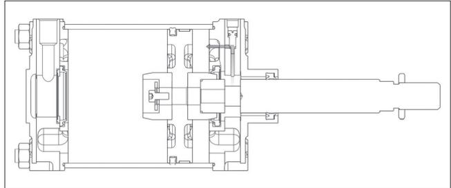
If cushioning is not provided then air passes through exhaust port only. When stroke comes to an end, piston strikes the end cover with some acceleration, giving rise to knocking noise, stresses on cylinder components and vibration transmitted to the machine structure.
