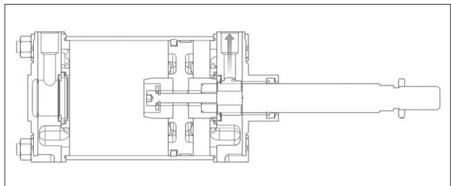
Perfect pneumatic cushioning produces minimal noise from end cover contact, and minimum piston deceleration time.
