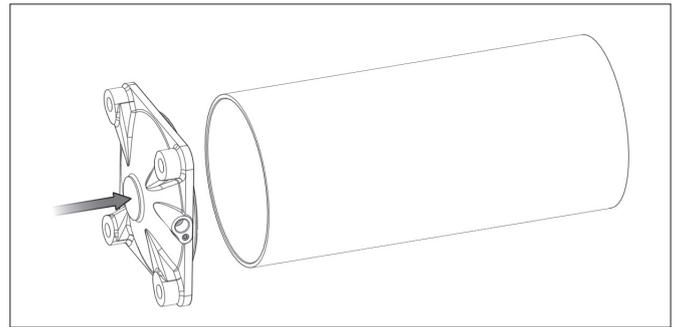
4. Assembled the cylinder cover nut (9) and tie rod (6) on rear cover (3) with tube (3).
