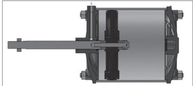
Perfect pneumatic cushioning produces minimal noise from end cover contact, and minimum piston deceleration time. To achieve perfect cushioning, ensure cushioning screw is full open at the time of installation. Operate cylinder in full forward to full back. Now keep on tightening cushioning screw till cylinder stops knocking. This will give maximum life to your equipment and to pneumatic cylinder.
