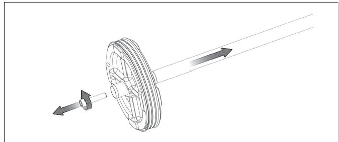
2. Remove lip seal (16) and buffer cap (10) from piston (4). Use blunt needle to remove lip seal (16).
