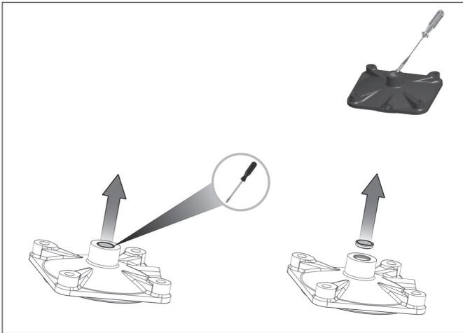
3. Remove o-ring (17) and cushion seal (15), take out cushioning screw (12) with o-ring (19) from front cover (1).
