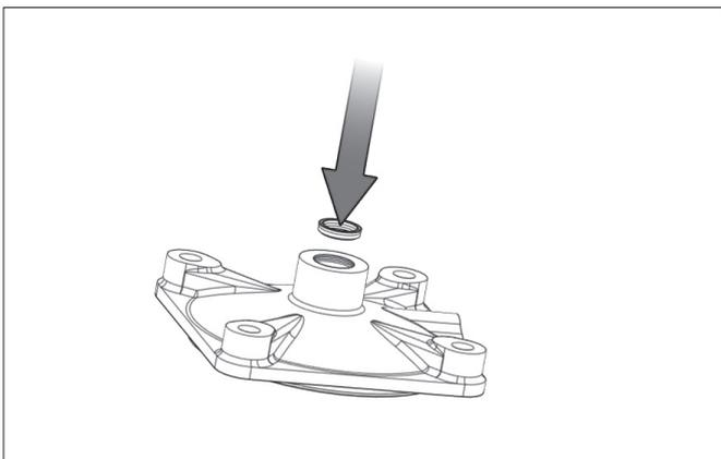
3. Place Cushioning seal (15) and o-ring (17) on its groove. Place o-ring (19) on cushioning screw (12), assemble the cushioning screw on rear cover (2).
