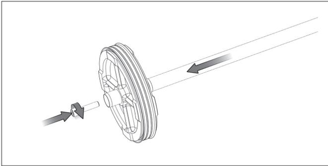
4. Insert this piston rod assembly carefully into the tube (3).
