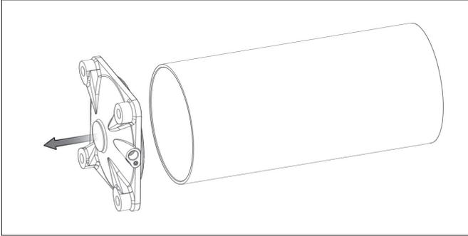
2. Remove o-ring (17) and cushion seal (15), take out cushioning screw (12) with o-ring (19) from the rear cover (2).
