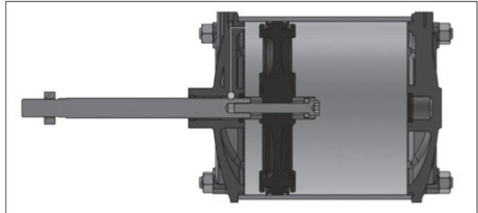
If cushioning is not provided then air passes through exhaust port only. When stroke comes to an end, piston strikes the end cover with some acceleration, giving rise to knocking noise, stresses on cylinder components and vibration transmitted to the machine structure.
