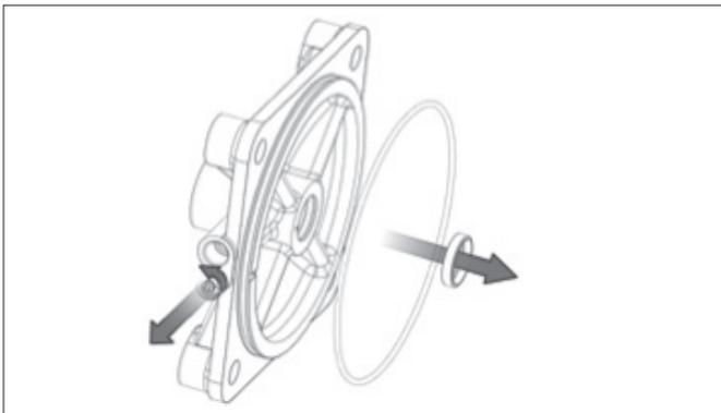
4. Clean it with liquid soap solution. After drying apply grease on
