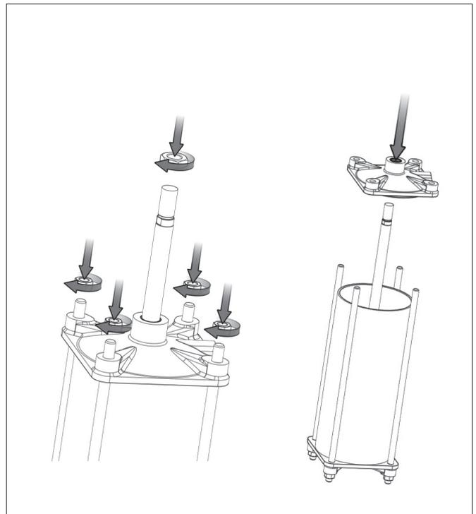
**NOTE:** Operate the cylinder assembly by hand. It should be free rotating piston rod & operating in and out.
