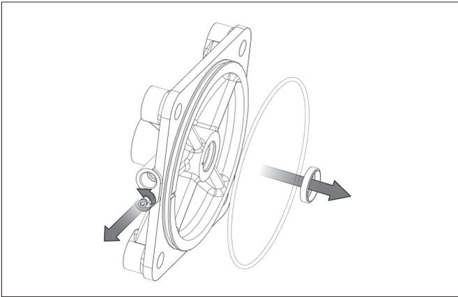
3. Clean tube (3) and rear cover (2) with liquid soap solution. After drying apply grease on rubber parts and inside the tube. Replace these rubber parts.
