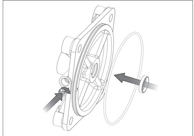
4. Assembled the front cover (1) on the tube (3), fasten the cylinder cover nut (9) and engage the lock nut (7).
